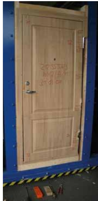
Tools used for testing 2nd security class doors.
